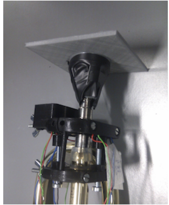
Figure 4. This figure shows an adapter (see also part no. 4 in fig. 2) mounted on the mouth piece of the trumpet to calibrate the sensor setup with defined weights. The sensor is an early prototype of the final setup shown in fig. 3. The trumpet is placed on a highly precise scale. The sensor is calibrated and the final accuracy is specified by putting different weights between 50 gr and 7 kg on the adapter fixed on the mouthpiece.
